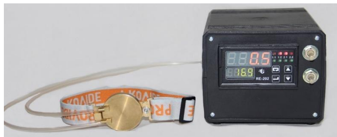
Fig. 2. Appearance of the device for contact cooling of the eye. Thermoelectric electronic cooling, control and power unit with cooling liquid heat exchanger [1].
