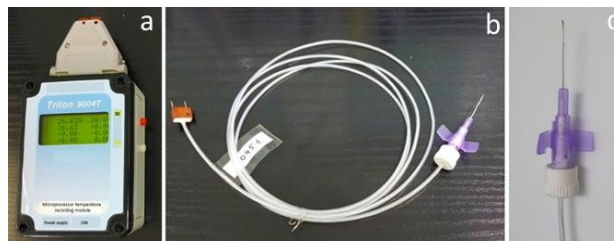
Figure 2. The thermoelectric device for measuring IOT. (a) microprocessor module for temperature data logging; (b) flexible thermocouple measuring probe; (c) measuring probe in a conventional polytetrafluoroethylene cannula housing (the outer diameter is 0.6 mm; its length is 19 mm) [2].
