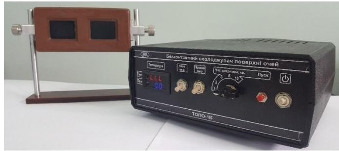
Fig. 3. Appearance of the thermoelectric medical device for contactless cooling of the eyes. Electronic control and power supply unit with thermoelectric cooling module [1].
